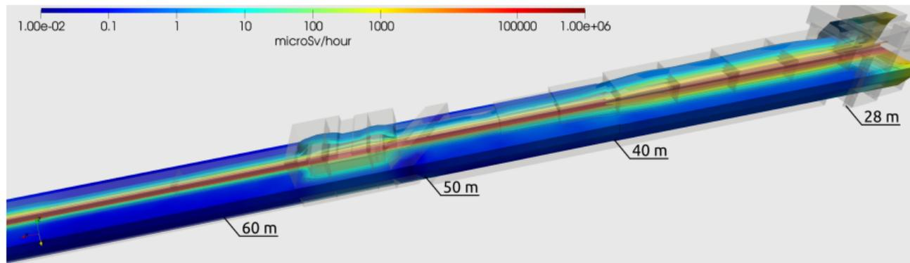
We show a detailed view of the Miracles shielding, 28 to 70 m. Translucent material represents an approximation to the shielding size of Miracles.
